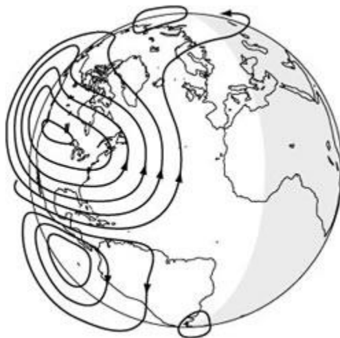
Fig. 2.7: Electric currents created in sunward ionosphere (Ionosphere - Wikipedia, the free encyclopedia.htm)
